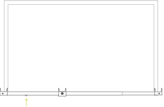
To determine the module length, rotate the spacing template, place the two outer spacing ribs against the module frame and tighten with the locking screw.
