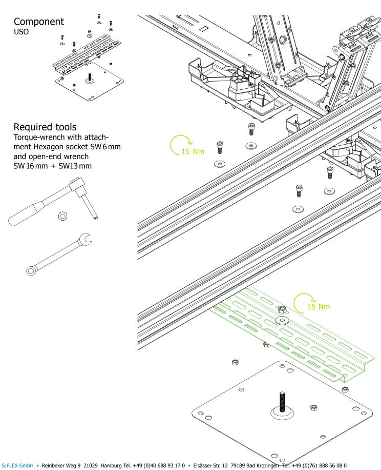
The USO attachment points are located on the Roll-bar Edge or Splice for roll-bar edge and should be fitted before the USO is assembled. The USO connection should be fixed as close as possible to a rail.
