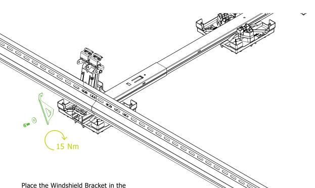
Place the Windshield Bracket in the position of a Tower Double+ on Windshield Connector and Windshield Edge.
