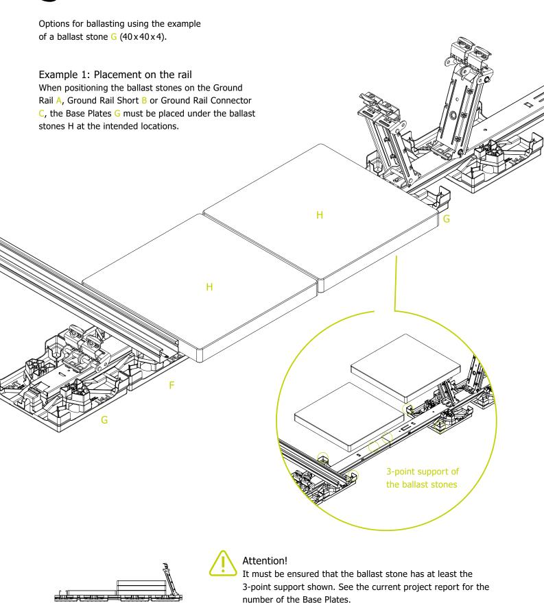
Optionally, depending on the insulation and size of the ballast stones, more Base Plates  ${\sf G}$  can also be installed.
